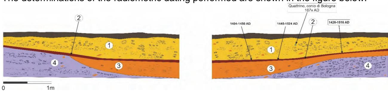
The reference number 1 indicates the lithological unit in which 3 debris flows are contained, indicated in the lithological profile of the trench (1st, 2nd and 3rd); the south wall on the left and the north wall on the right.
