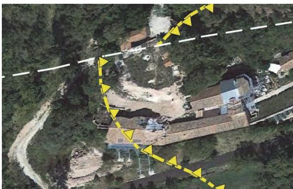
The yellow dotted line indicates a thrust fault and the white dotted line indicates a right transcurrent fault.
